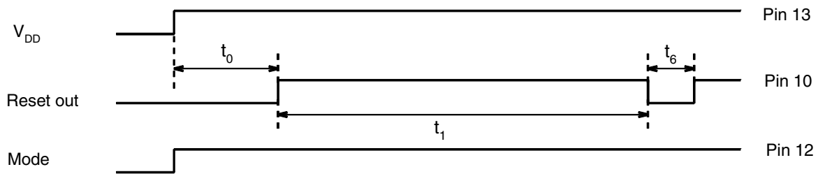
Figure 4-2. Power-up Reset and Mode Switchover
